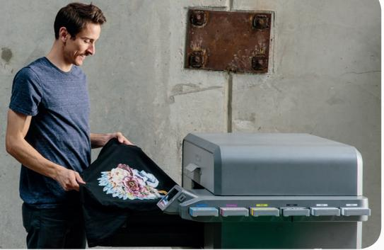
DTG (Direct to Garment) is a relatively new garment printing technology. It uses purpose designed inkjet printers, such as Ricoh's Ri 3000 and Ri 6000, to apply water-based pigment inks directly to cotton and cotton/polyester mix garments. Because the process is digital, the design can be changed from one garment to the next.
