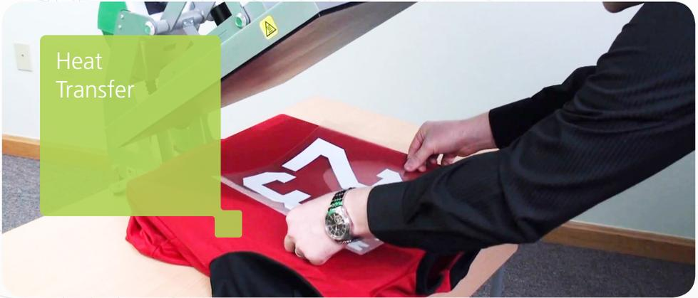
Images are printed onto specialised heat transfer paper using a laser printer and transferred to the garment using a heat process. The process supports local production and personalisation (like Inkjet DTG) but can be fiddly as images must be printed in reverse, the heat transfer paper has to be trimmed before the image is applied and specialised paper is required to apply a white underlay.
